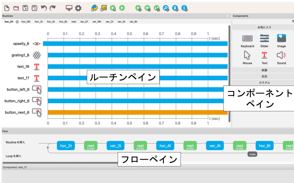
Figure 3-3 PsychoPy Builder experiment creation screen. It consists of three panes, where the stimuli etc. selected in the component pane are placed in the routine pane, and the order of the routines is determined in the flow pane.
